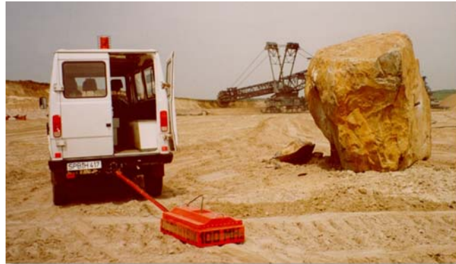
Figure 9: Georadar measurement in an open-pit mine
