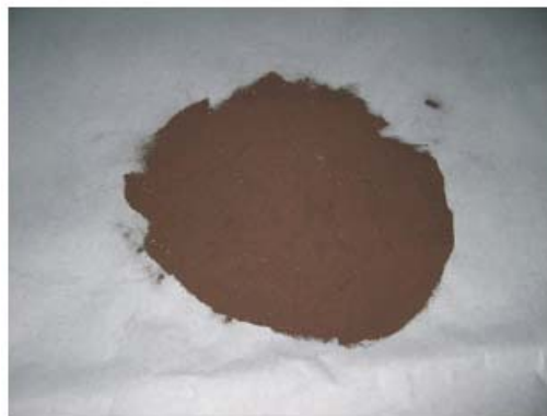
Figure 7 The aspect of the roasted pyrite at 400°C
