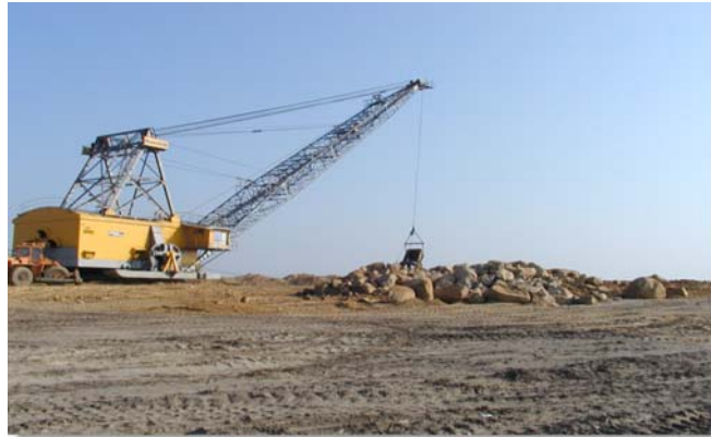
Figure 12: Dragline excavator to extract stones and rocks
