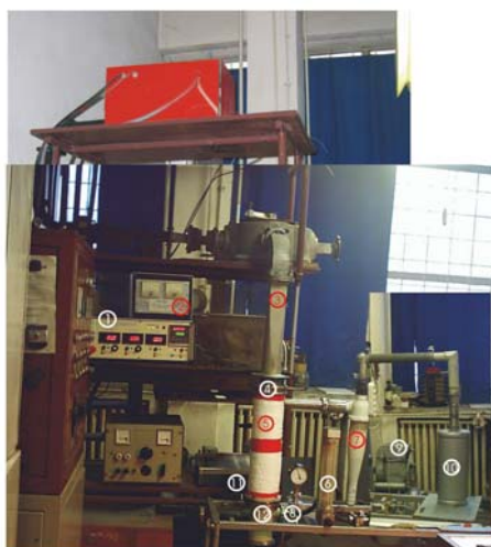
Figure 2- The microwave heating installation in fluidized bed.
