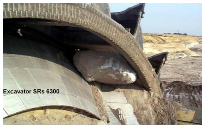
Figure 4: A rock wedged in the bucket wheel of an SRs 6300
